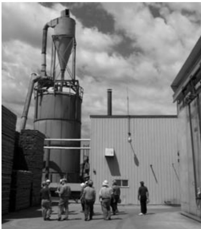
At a tour of Hawkeye Forest Products in June, 2006, with kilns on one side and stickered stacks of lumber on the other, the tour group observes the storage tower for planer shavings that are used as fuel to heat the kilns.
