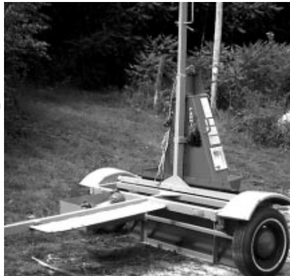
The Farmi is tipped up, ready to mount on a tractor. It is transported laying horizontal on this custom trailer built by Paul Bader.
